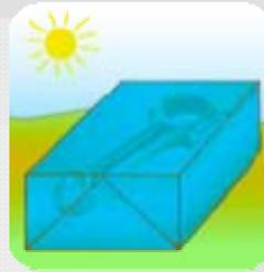
More tight packaging means less VCI loss during the shipment. Holes can be fixed with tape with no influence on VCI effectivity.
