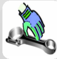
Always use gloves when dealing with parts to be packed after final cleaning stage. Human sweat contains basic acids which can be very corrosive in certain conditions.
