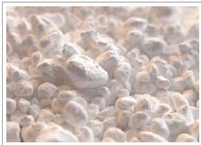
I granuli del FerroFlam MCA granule misurano 0.4-0.5 mm
